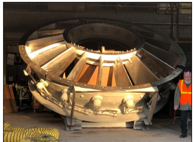
Horizontal Kaplan cast iron distributor. Repaired with over 600 pounds of machinable super-nickel overlay applied without welding.
